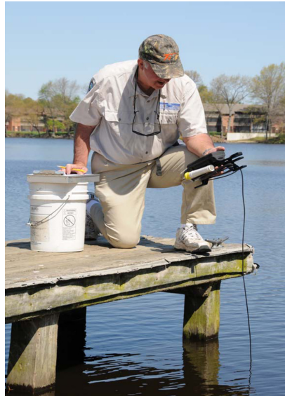
ECSI scientist, John Foster, uses the YSI ProODO optical handheld DO instrument, attached to the cable management kit, to measure water quality in high hydrogen sulfide environments.
